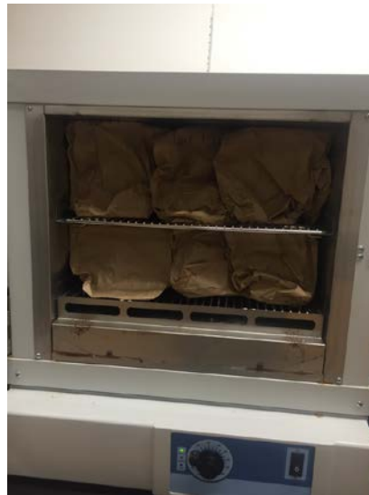
Figure 6. Biocontainer samples placed in drying oven for forty-eight hours at 60°C.
