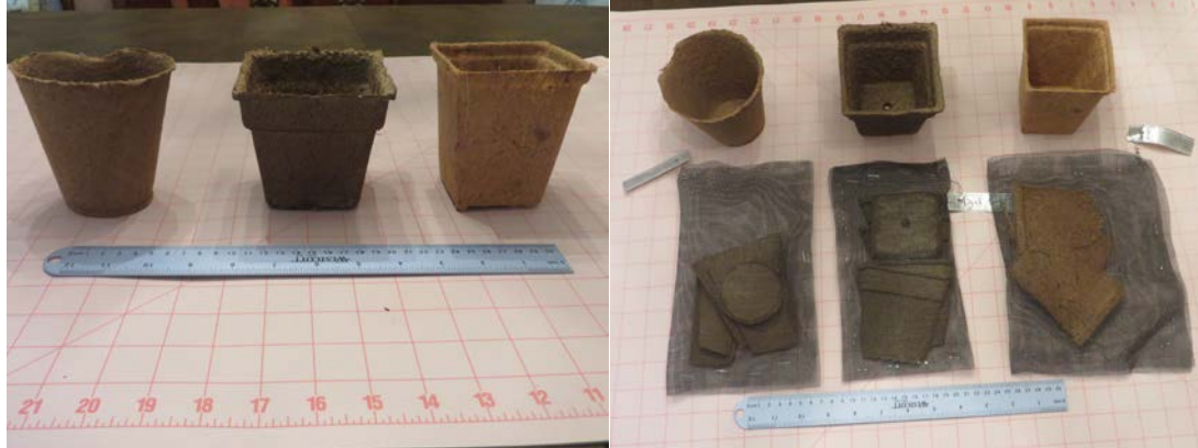
Figure 1. Cowpot, Fertilpot, and Coconut Coir pot containers placed in mesh bags designed from mesh fiberglass screen.
