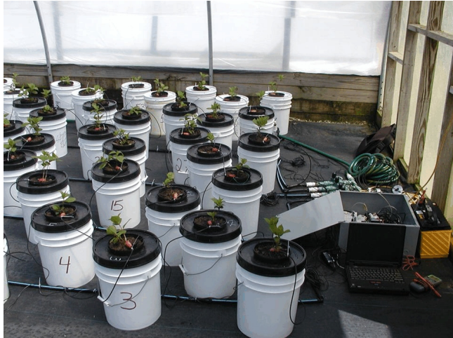
Picture 1. Plants were placed in the lids of 5-gallon buckets so that the leachate collected in the buckets. A datalogger (in the metal enclosure on the right) controlled solenoid valves, allowing for precise control of the substrate moisture level in five different treatments. The datalogger was connected to a laptop computer, allowing us to monitor the data.
