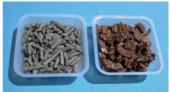
Figure 4. Examples of pelletized and processed and colored recycled newspaper that can be used as mulch. Credits: Robert H. Stamps
